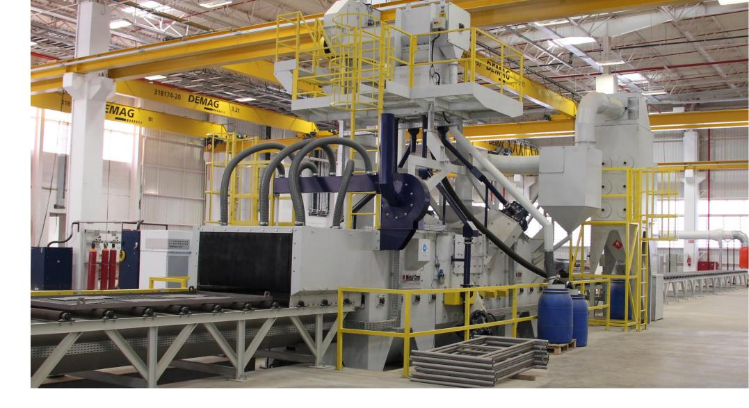
Cym Materiales SA manufactures continuous flow equipment for **shot blasting welded structural shapes, profiles, bars, plates, steel strips and pipes** according to the needs of each customer.
